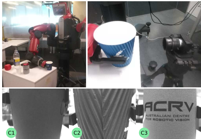
Fig. 1. Interactive, Visual Analysis of an Object’s Material Properties. Baxter squeezing a range of items (top-left), with an external camera observing (top-right). By applying a known, periodic stimulus, we show that matched video filtering and simple statistics can be used to distinguish objects based on material properties, even for stiff, fragile, or low-texture objects. (bottom) Example input frames for three beverage container types: C1 has little texture, C3 shows only small deformations, and C1 and C2 are easily crushed.
