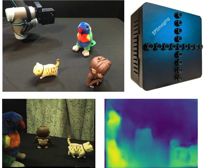
Fig. 1. We propose an unsupervised approach to interpret new imaging devices like the EPIModule from EPIImaging LLC shown here. We propose a novel encoding scheme that benefits from the view diversity of these devices while allowing a broad family of cameras to be used without manual intervention. To demonstrate the technique we learn visual odometry and depth estimation, delivering metric results with greater accuracy and detail than prior approaches.
