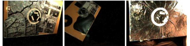
Fig. 5. Example of images from the data collected with our satellite docking test bench and the Davis 346 RGB/event camera. (a) and (b) are from the *augmented texture* training set. (c) is from the *realistic training* set.
